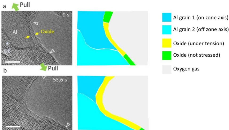
Fig.1. Sequential TEM images showing the super-elongation and self-healing process of aluminum oxide when stretched in O<sub>2</sub> environment<sup>1</sup>. Oxide between the two white triangular marks in (a-b) are the segment being stretched (also highlighted as yellow color in the schematic drawings). The green arrow in (a) represents the stretching direction. The strain of oxide at (b) is about 117%. All scale bars, 5 nm.
