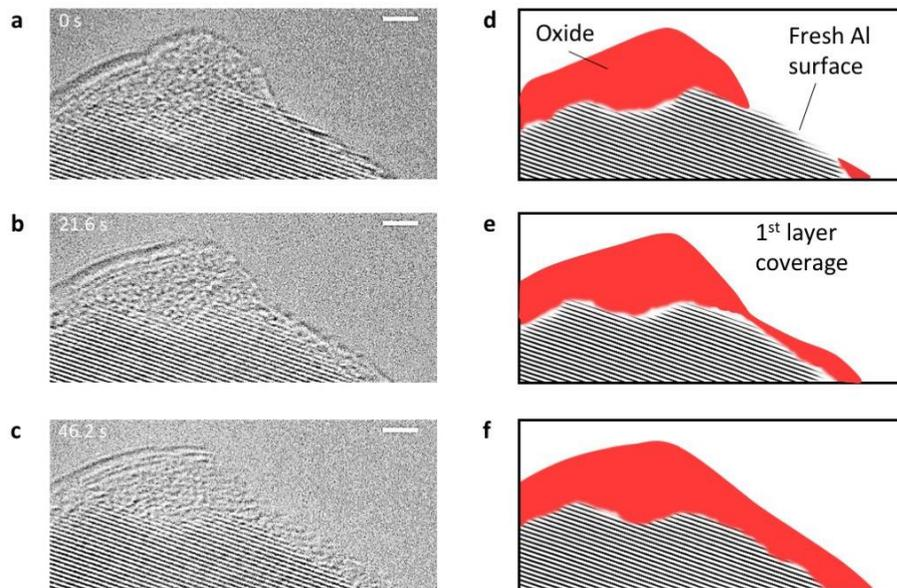
Fig. 2. Initial oxidation of pure aluminum at room temperature<sup>1</sup>. a-c, Sequential HRTEM images of the oxidation process. d-f, processed images of (a-c) to highlight different phase distribution: the aluminum lattice planes, shown by black lines, are filtered images of (a-f) using a set of aluminum (111) diffraction spots; the oxide is shown by red color. All scale bars, 2 nm.
