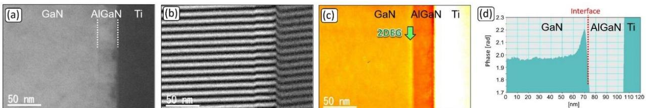
Figure 1 (a) TEM image, (b) hologram, (c) reconstructed phase image, (d) phase profile around GaN/Al<sub>0.25</sub>Ga<sub>0.75</sub>N sample.
