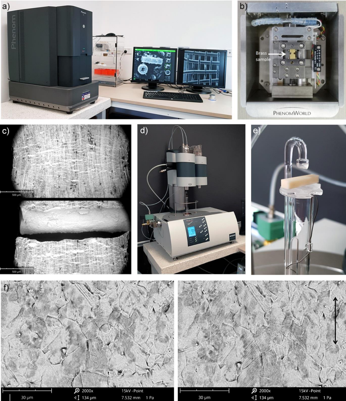
Figures a – f : a) The Phenom XL SEM located at the AMCF, b) the In-situ SEM tension stage with a brass sample sitting in the centre, c) In-situ SEM images of an unpolished brass sample before and after fracture, d) the Netzsch TMA setup, e) TMA setup for a three point bend test and f) In-situ SEM images of an etched brass sample before tension (left) and under tension (right). Here the grain boundaries can be seen. As the sample is put under tension, stretching of the grains can be seen as well as the appearance of micro-fractures (black arrow shows direction of tension).
