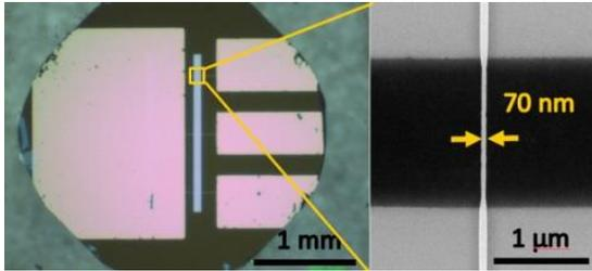
Fig. 1 Left: Si chip mounted with Gold electrodes and pads.
