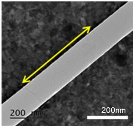
Fig. 2 TEM image of the Graphene Nanoribbon
