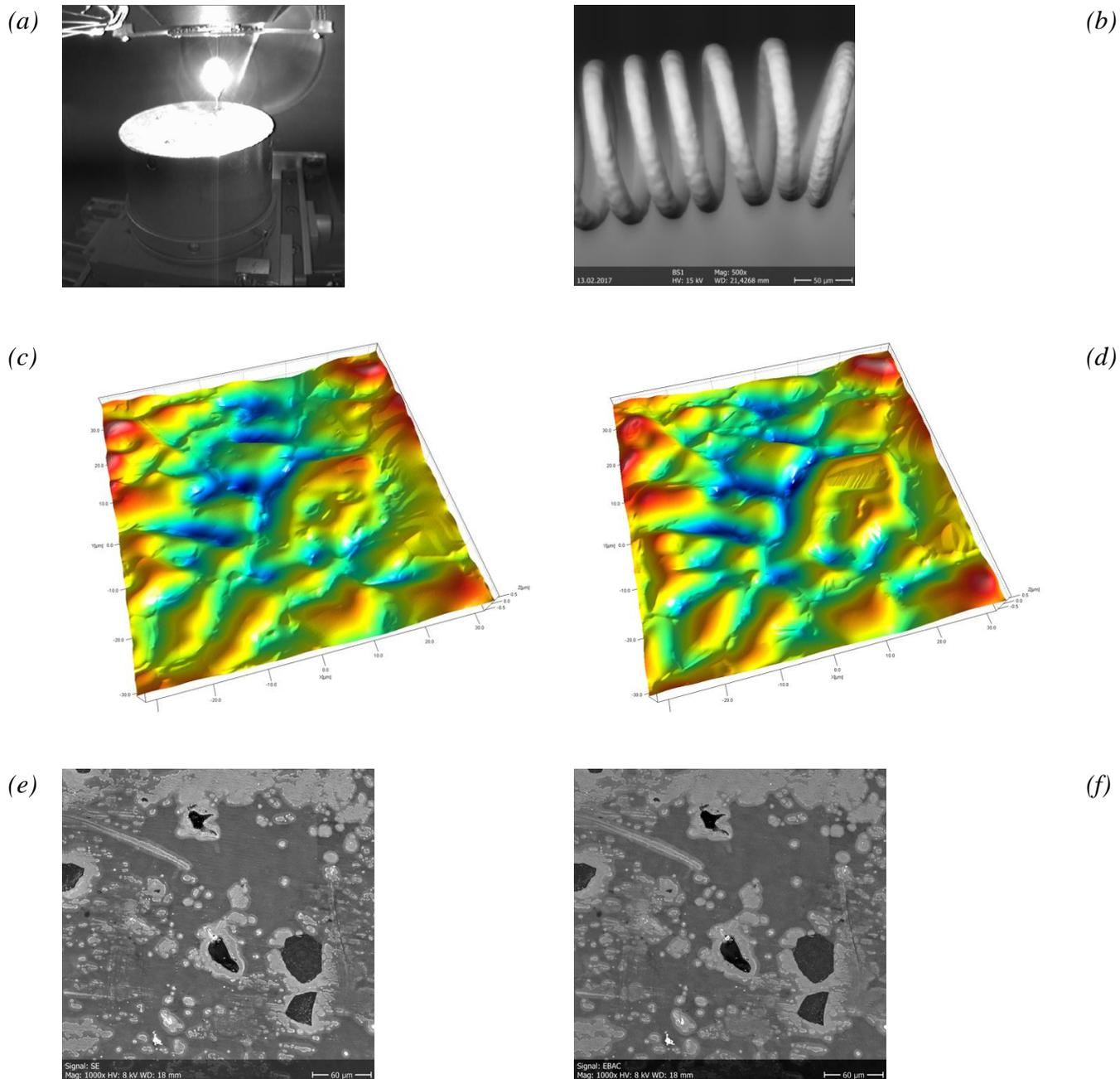
**Figure 1.** IR chamberscope view of heated W filament **(a)** and corresponding HT BSE image **(b)**. Extracts from a time series topographic reconstruction of Cu catalyst during hydrogen oxidation **(c, d)**. Large field detector **(e)** and Electron Beam Absorbed **(f)** images of graphene on Pt at 400 °C.
