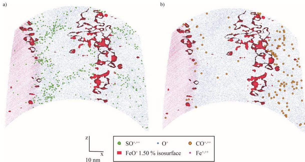
Figure 1: a) and b) are the same 4 nm section extracted from an atom probe dataset, where the Fe-20Cr substrate can be seen on the left of each image. a) shows the SO<sup>+</sup> and SO<sup>++</sup> ions, which are distributed throughout the inner and outer oxide grain boundaries. b) shows the CO<sup>+</sup> and CO<sup>++</sup> ions, which are situated predominantly within the outer section of the oxide scale.
