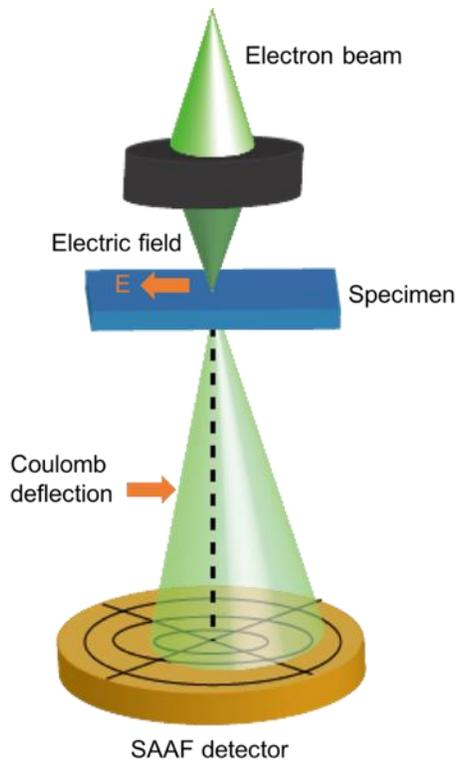
Fig. 1 Schematic image of DPC STEM.
