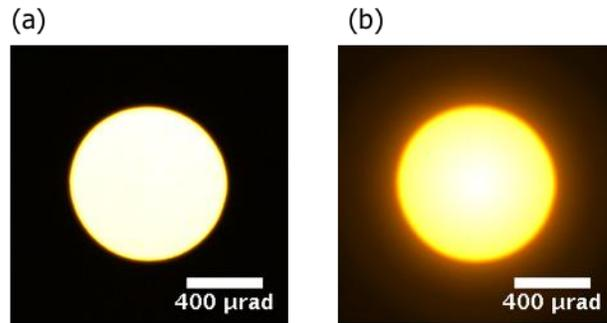
Fig. 2 (a,b) Bright field disk patterns of without and with specimen, respectively.
