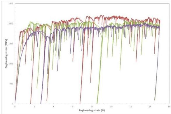
Fig.1: Engineering stress-strain curves of micro-pillars subjected to in-situ compression tests (three different tests were carried out on micro-pillars of similar dimension to ensure reproducibility).
