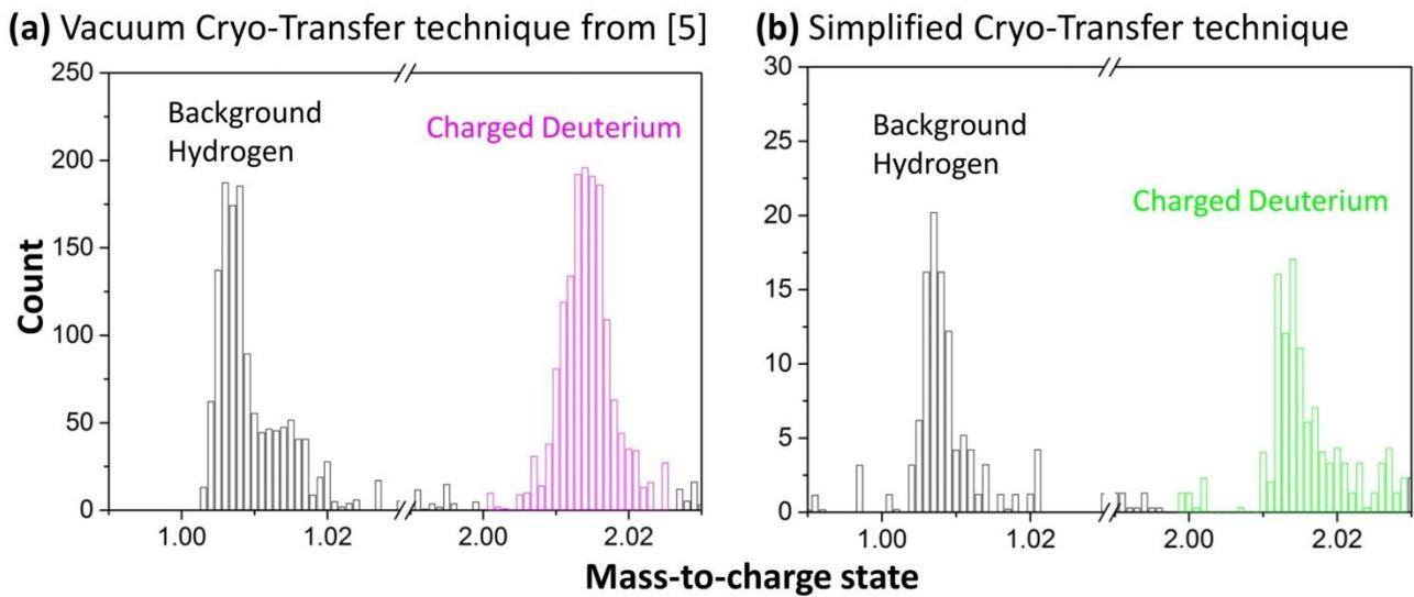
Figure 2. Comparison of the resulting global deuterium content in a ferritic sample containing 10-20nm fine V-Mo-Nb carbides as hydrogen traps from both cryo-transfer approaches.
