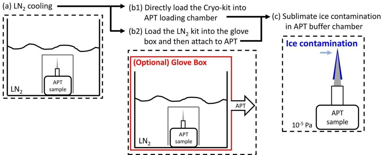
Figure 1. Experimental configuration of non-vacuum cryo-transfer technique
