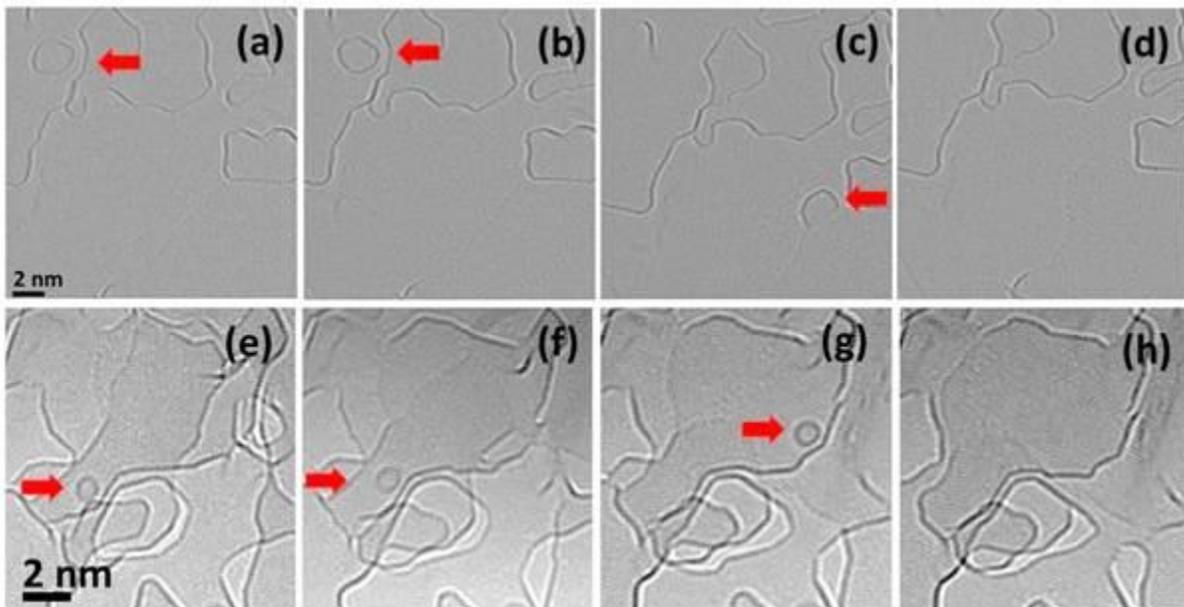
Figure 2: (a-d) Migration and merging of a graphitic flake at 1200 C and (e-h) movement of a cage like structure at 1200 C.
