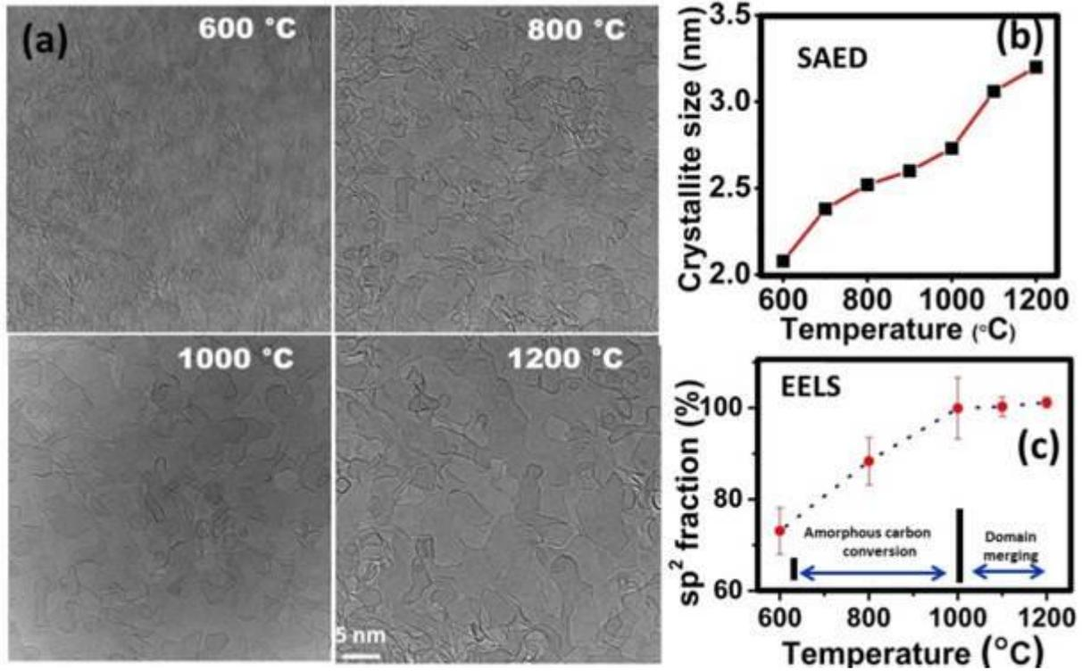
Figure 1: (a) The evolution of domains, (b) crystallite size evolution during heating and (c) the sp<sup>2</sup> carbon content at different temperatures. The sp<sup>2</sup> content increases from 600 C to 1000 C and saturates indicating that the amorphous sp<sup>3</sup> carbon is completely consumed at 1000 C and further domain growth is facilitated by merging of domains.
