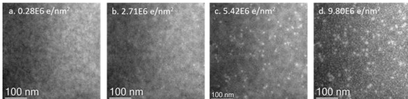
Figure 2: EFTEM images obtained at an energy loss of 17 eV showing the Si nanoparticle formation. Dose rate:  $\sim 55000$  e/nm<sup>2</sup>.s.
