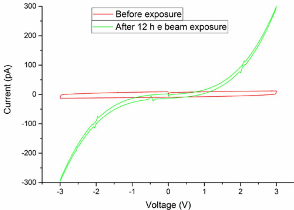
Figure 1: Electrical conductivity of a 15 nm thick SiO<sub>2</sub> thin film before and after exposure to the electron beam with a total dose of  $3 \times 10^7$  e/nm<sup>2</sup>. The I/V curves were recorded with the electron beam off. Dose rate  $\sim 500$  e/nm<sup>2</sup>.s.
