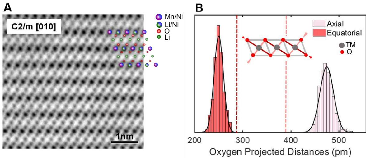
Figure 1. High-resolution STEM-ABF image of pristine  $\text{Li}_{1.2}\text{Ni}_{0.2}\text{Mn}_{0.6}\text{O}_2$  viewed along the  $C2/m [010]$  zone axis (a). Histograms and fitted Poisson probability density functions of the axial and equatorial O-O bonds in charged LNMO (b). Dashed lines indicate the mean projected interatomic distances for the pristine material.
