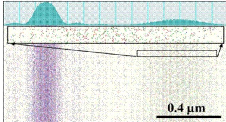
Fig. 2. Composite image of color-coded electrons of present version of the "which-way" double-slit experiment: blue colored electrons passed through only the left slit; red colored electrons passed through both slits simultaneously; green colored electrons passed through only the right slit. Inset is an averaged intensity profile of the pre-Fraunhofer fringe pattern. The second inset indicates an enlarged figure of the data in the rectangle area shown below.
