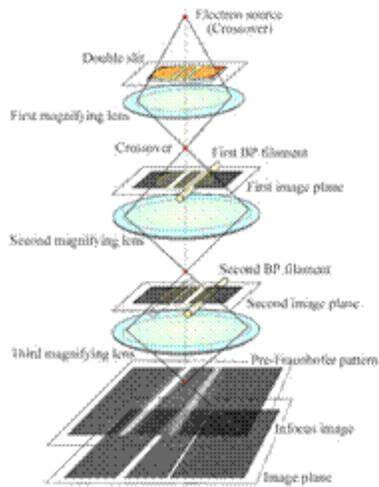
Fig. 1. Schematic diagram of optical system. The double slit and two electron biprisms are placed at the conjugate planes in the system. The resultant asymmetric double-slit image is observed in pre-Fraunhofer condition.
