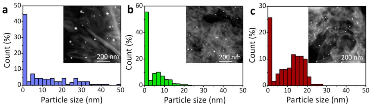
**Figure 1:** Co-catalyst particle size distributions of used 5 wt% Pt/g-CN's: (a) g-CN:1, (b) g-CN:2, and (c) g-CN:3. Insets depict representative ADF-STEM images of each photocatalyst.
