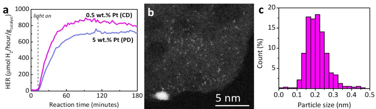
**Figure 2:** (a) Hydrogen evolution rates for two different Pt loading methods on g-CN:1. (b) ADF-STEM image of fresh 0.5 wt% Pt/g-CN:1 and (c) corresponding Pt particle size histogram.
