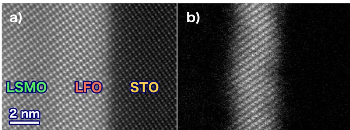
Figure 1: Atomic resolution pixelated STEM imaging: a) HAADF image; b) image from the intensity in the innermost HOLZ ring.
