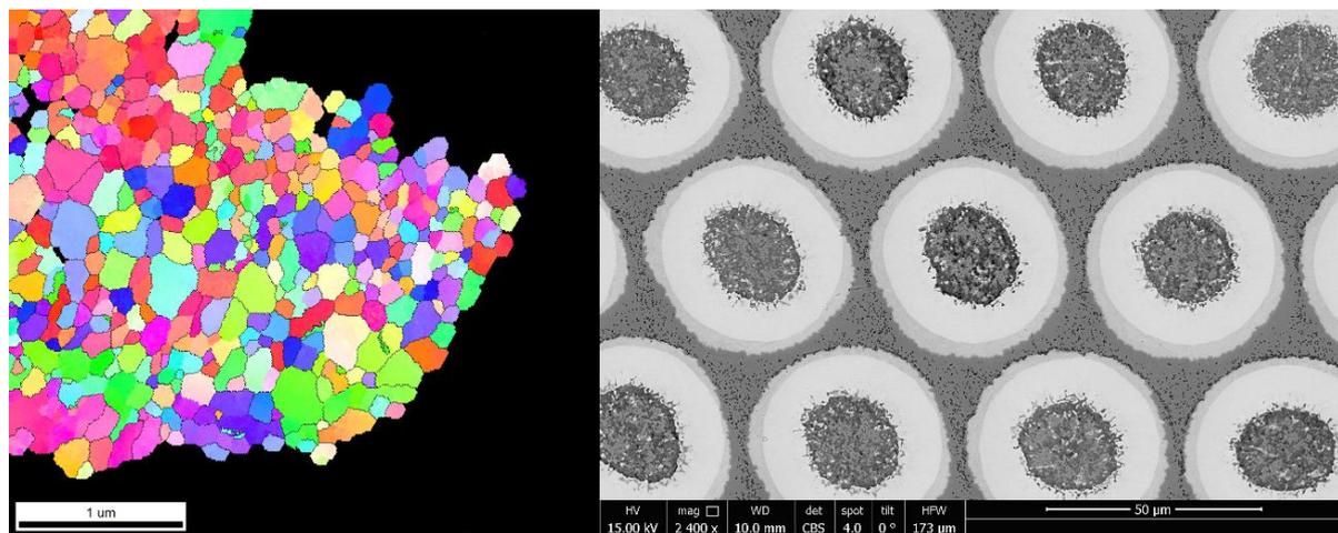
TKD inverse pole figure map of a TEM specimen (left) and SEM image of the cross section of a powder-in-tube (PIT)  $\text{Nb}_3\text{Sn}$  superconductor (right).
