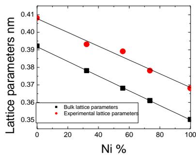
**Figure 2:** Lattice parameters plot as a nickel percentage function highlight a Vegard's law as found into bulk alloys. However, one can observe a 4 % decrease of the NPs lattice parameters unambiguous associate with surface effects.
