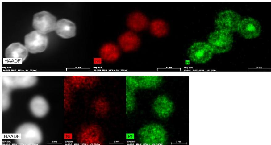
**Figure 1 :** HAADF-STEM (High resolution high-angle annular dark-field imaging) NPs of (top)  $Ni_3Pt$  core-shell image where Pt presents a stronger contrast than Ni and (bottom) an uniform  $Ni_3Pt$  NPs contrast which are confirmed by local EDX - Ni (K line) and Pt (M line) chemical mapping
