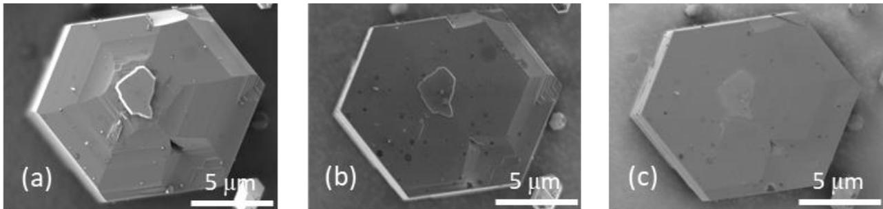
Figure 2. (a) strong topographic contrast in the image from the E-T detector, (b) material contrast from the Multidetector, (c) surface-sensitive material contrast from the Axial detector.
