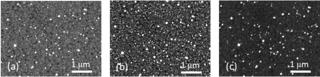
Figure 1. (a) topographic and Z-contrast in the image from the in-chamber BSE detector, (b) Z-contrast from whole interaction volume from the Mid-Angle BSE detector, (c) Z-contrast from a thin surface layer from the In-Beam BSE detector.
