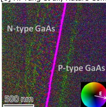
Figure 1. Electric field map of the PN junction in GaAs.
