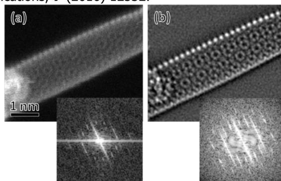
Figure 2. (a) ADF image and (b) ptychographically reconstructed phase image of SWCNT.
