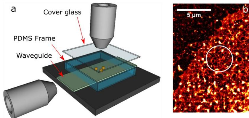
*Figure 1: (a) Schematic overview of the chip-based nanoscope. A coupling lens (far left) couples light into the waveguide. The light is guided along the waveguide and excites samples in contact with the surface (yellow spheres) through the evanescent field. A hollow PDMS frame is used to contain the sample and blinking buffer. The area is sealed off with a cover slip and the sample is imaged from the top using a*
