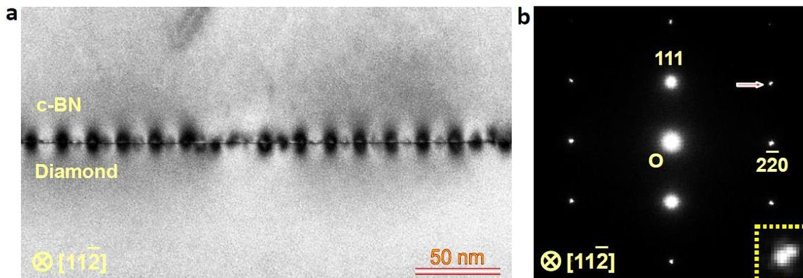
Fig. 1. Microstructure of the {111} diamond/c-BN interface. (a) Bright field TEM image and (b) corresponding diffraction pattern.
