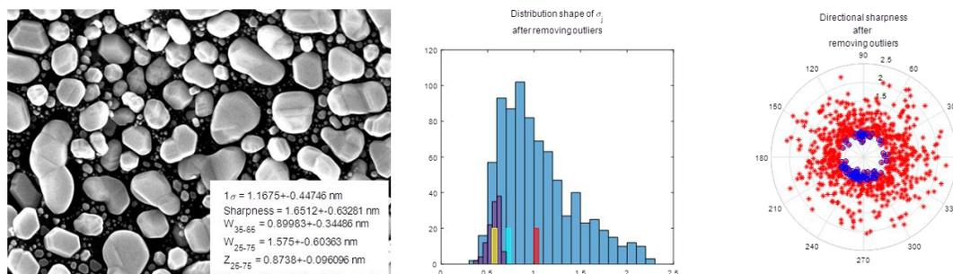
Fig. 2. Image sharpness measurement using derivative method.
