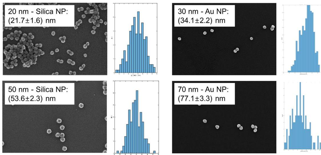
Fig. 3. SEM measurement results for silica and gold nanoparticle size.
