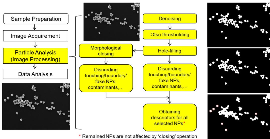
Fig. 1. Procedure for NP size measurement using SEM.
