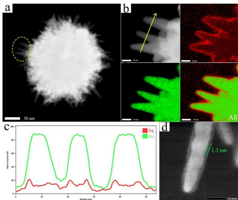
Fig. 1(a) HAADF-STEM image of urchin-like gold NPs (b) EDS mapping of the selected region showing elemental distribution of Ag , Au and their overlay; (c) EDS elemental linescan taken along the yellow line in (b) to demonstrate the elemental composition of nanotips; (d) HAADF-STEM image of nanotips to demonstrate the thickness of the alloy layer.
