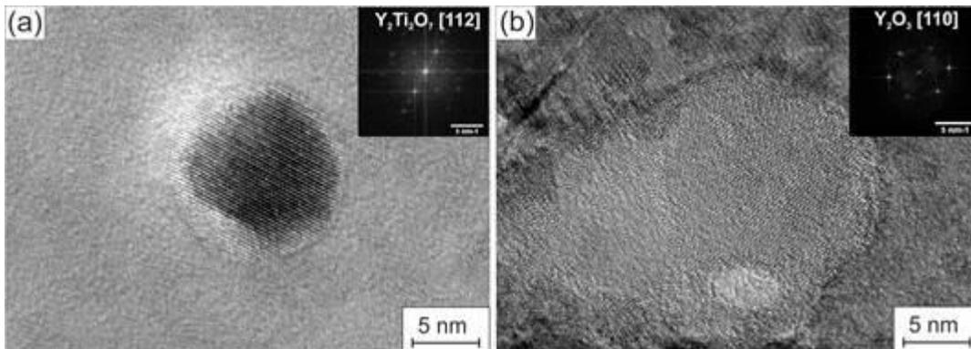
**Figure 2.** HRTEM images of ODS particles with corresponded diffractograms
