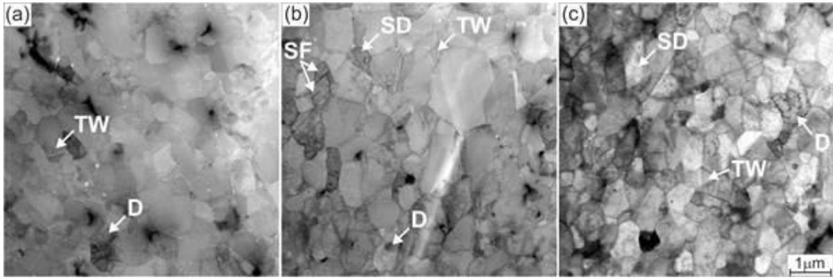
**Figure 1.** Inverted contrast HAADF-STEM micrographs reveal microstructures (a) before (as-received state) and (b) after cyclic straining at 650°C under  $\pm 0.4\%$  and (c) under  $\pm 0.7\%$  strain amplitude. By arrows are marked: D - dislocations, TW- twins, SD - short dislocations or loops, SF - stacking faults.
