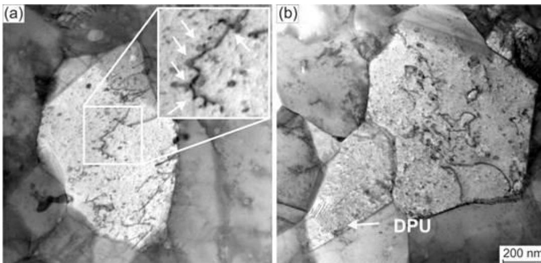
**Figure 3.** Inverted contrast HAADF-STEM micrographs revealing dislocations structure after cyclic straining at 650°C under  $\pm 0.4\%$  (a) and  $\pm 0.7\%$  (b) strain amplitudes. Insert in (a) shows pinned dislocation at various nanoparticle-matrix interfaces (arrows). In (b) by arrow is marked dislocations pile-up (DPU).
