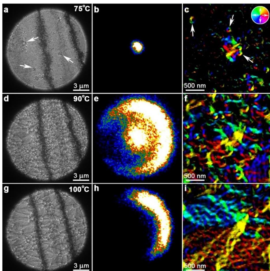
**Fig. 2** (a,d,g) Fresnel; (b,e,h) SAES; and (c,f,i) pixelated DPC images of an HF-etched FeRh thin film acquired during *in situ* heating to (a-c) 75°C; (d-f) 90°C; and (g-i) 100°C. The images demonstrate the different stages of the magnetostructural transition, including (a-c) nucleation of magnetic vortices (arrowed); (d-f) AF / FM phase co-existence; and (g-i) a fully FM state. The direction of magnetization in the DPC images is depicted in the colour wheel (Fig. 2c, inset).
