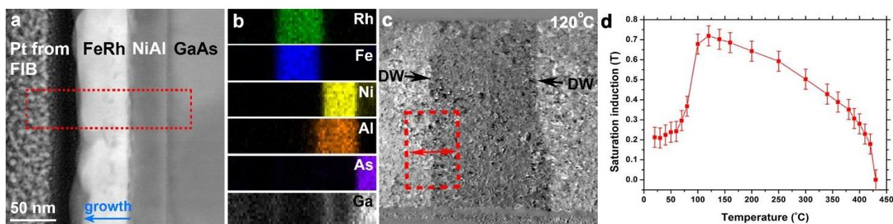
**Fig. 1** (a) STEM image of an FeRh thin film epitaxially grown on a NiAl buffer layer and GaAs substrate. (b) EDS spectrum image acquired from the boxed region in (a), and chemical maps showing their elemental content. (c) DPC image of magnetic domains/DWs in a planar FeRh thin film acquired at 120°C. (d) Graph of saturation induction as a function of temperature, calculated using direct measurements of electron-beam deflection from the DW in the boxed region (red) defined in (c).
