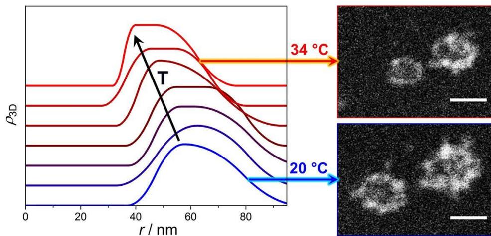
**Figure 1:** Temperature-dependent collapse of a PNIPAM-based microgel stained with AgNPs. Reprinted with permission from [3]. Copyright 2016 American Chemical Society.
