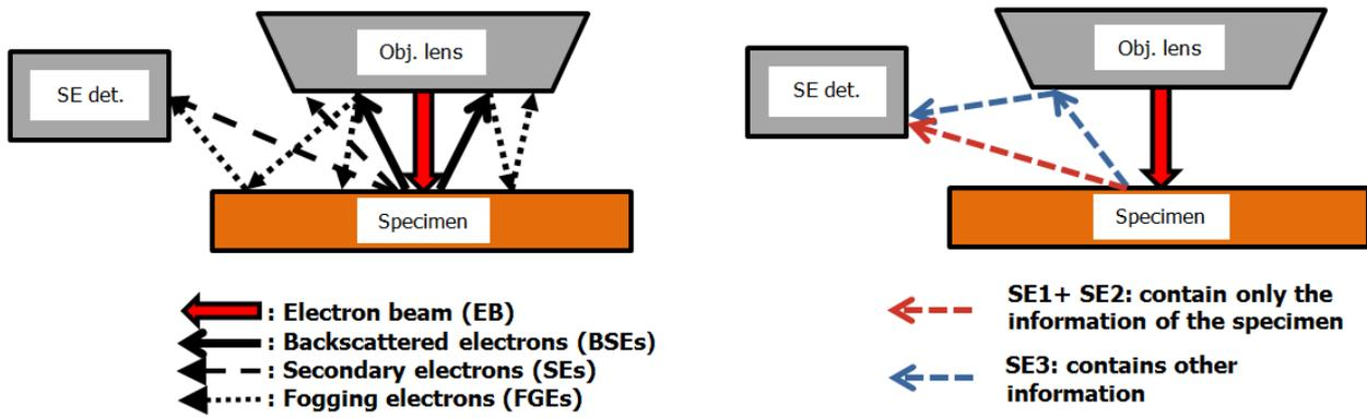
Fig. 1 The Schematic diagram of FGEs and detected electrons by the SE detector.
