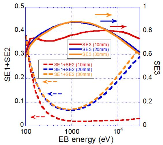
Fig. 3 SE detection ratio.
