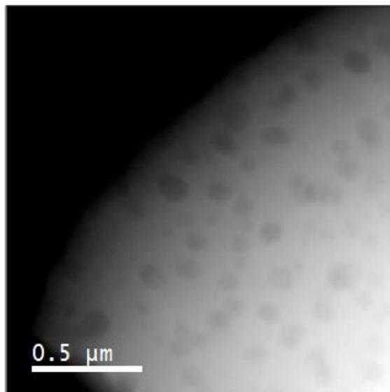
**Fig. 2** ADF-STEM image of phase-separated glass
