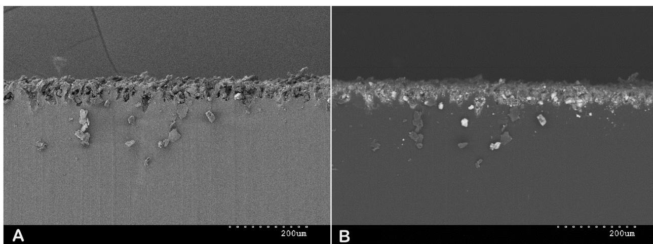
Fig. 1. Secondary electron image (A) and backscattered electron image (B) of a polymer jacket.
