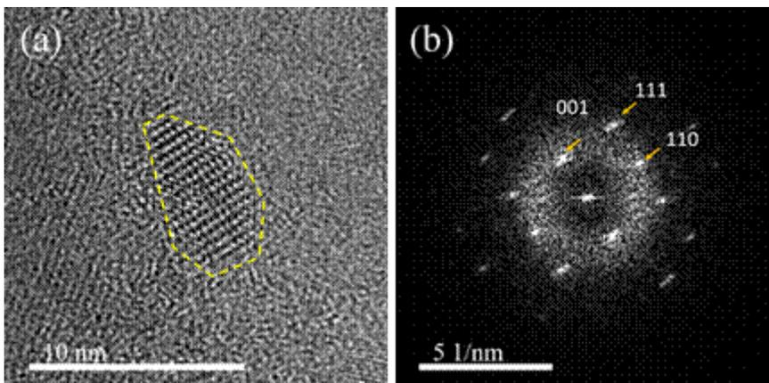
**Figure 2.** TEM image of AgI particle and its FFT pattern.
