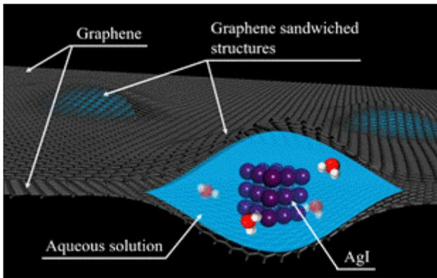
**Figure 1.** An illustration of water encapsulated inside graphene sandwiched structure.
