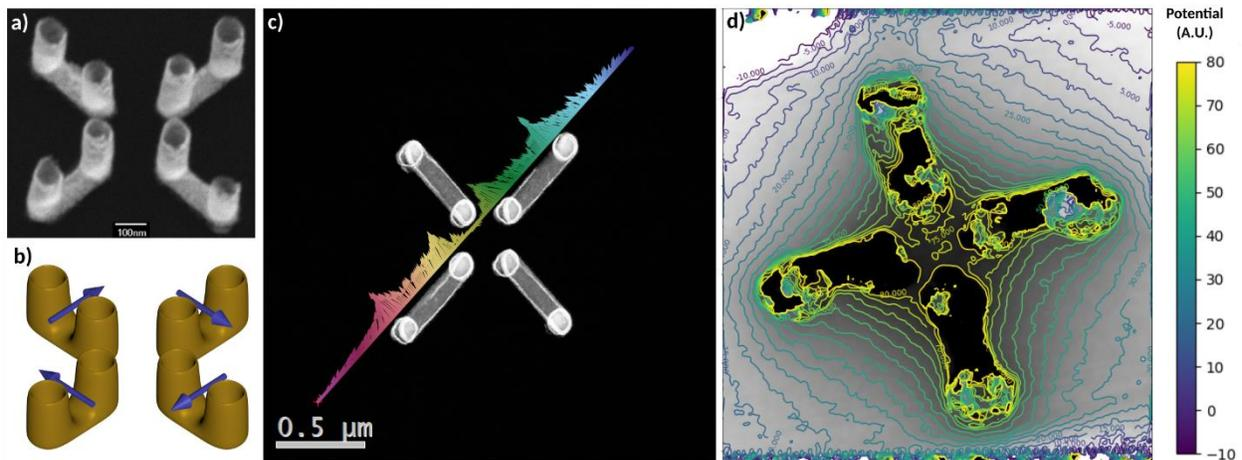
**Figure 1:** a) SEM electron micrograph highlighting a typical toroidal nanostructure. b) Schematic diagram of the toroidal nanostructure with the expected in-plane magnetic field (purple arrows) of the toroidal dipole moment. c) DPC line profile recorded near the toroidal nanostructure. The arrows represent the deviation (not to scale) of the electron beam from the optical axis. d) Potential map in arbitrary units calculated from an EH recorded on the toroidal nanostructure.
