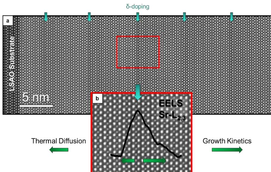
**Figure 1.** (a) STEM-HAADF image of a Sr  $\delta$ -doped heterostructure exhibiting high structural quality. (b) Larger magnification of the area highlighted by the red rectangle in (a). The inset shows the integrated Sr- $L_{2,3}$  EELS line profile presenting an asymmetric dopant distribution.
