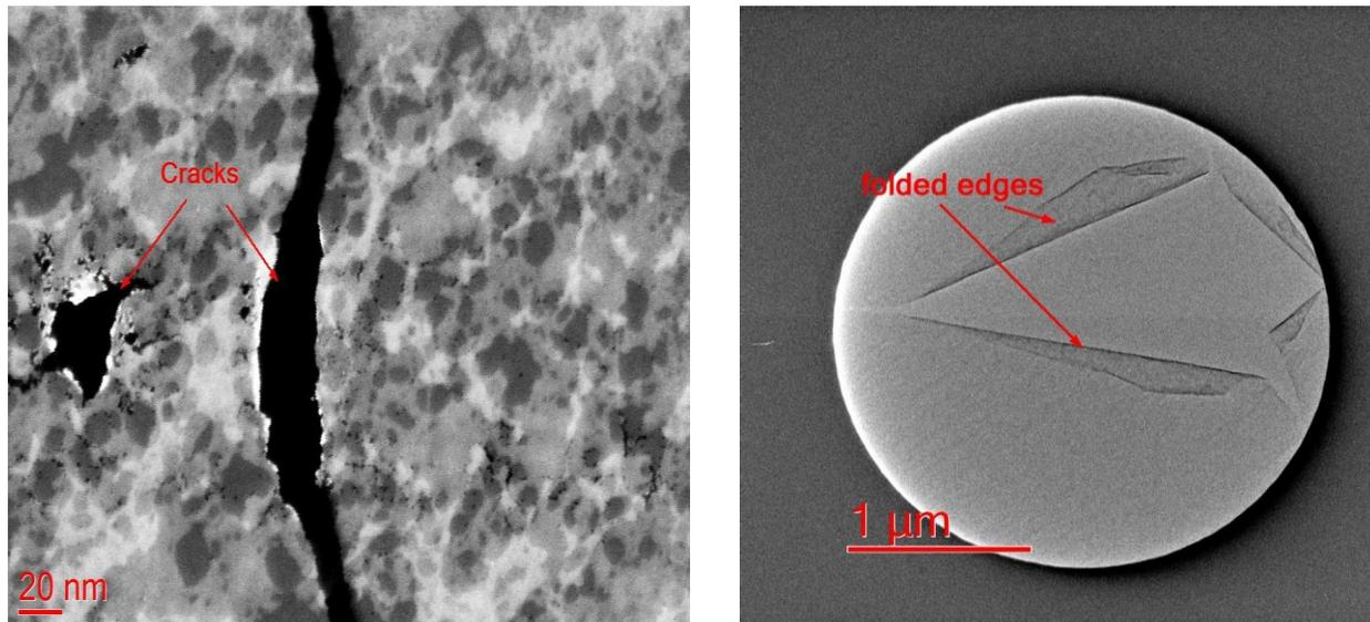
Fig. 1 (left): Production of holes and cracks at the nm-scale on WSe<sub>2</sub>-monolayers. In order to cut and investigate holes inside the monolayer STEM HAADF was used.
