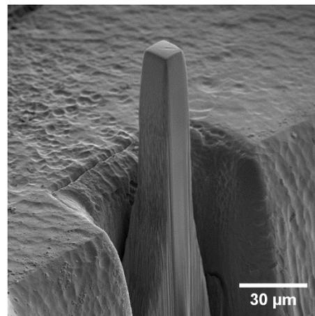
Fig. 1 Fabricated micropillar with a diameter in the range of a few μm for testing the size limits
