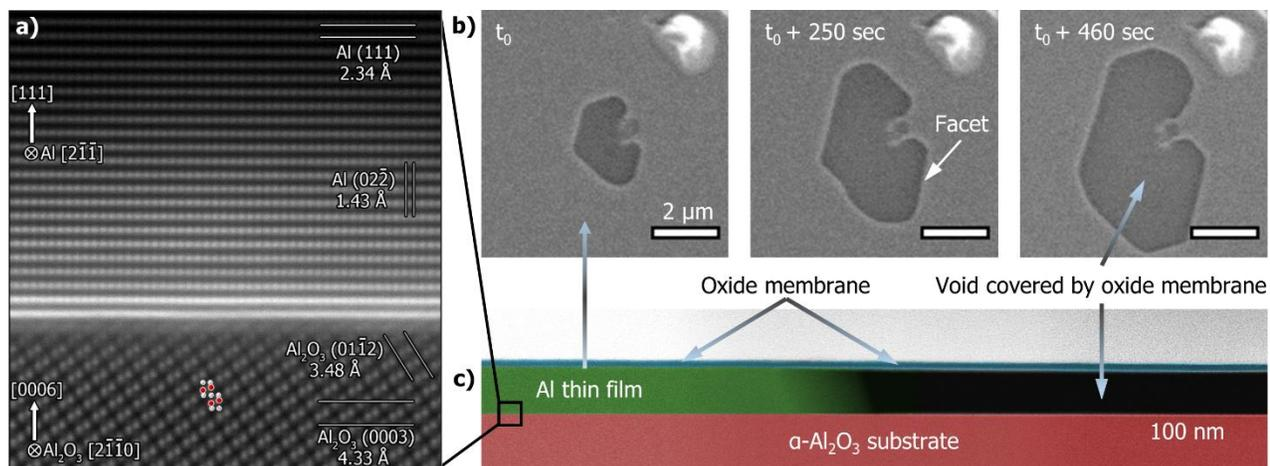
**Figure 1:** a) Atomic resolved STEM micrograph of a region adjacent to the Al|void interface confirming OR a/b (overlay: Al red, O white). b) Evolution of a faceted void while annealing in the ESEM at 500 °C in oxidizing atmosphere. c) The cross-sectional color-coded HAADF STEM image shows a continuous alumina membrane (bright blue) covering both, the void (black) and the film (green).
