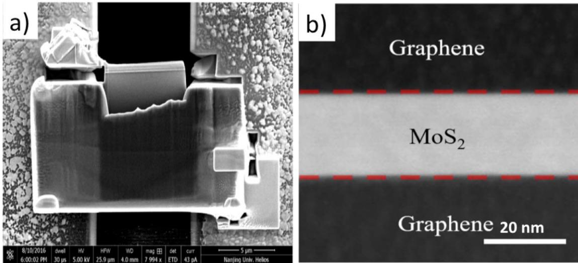
**Figure 1.** (a) (c) In-situ GMG device sample welded on a home-made in-situ electrical biasing chip. (b) Cross-section HAADF image of a pristine GMG device.
