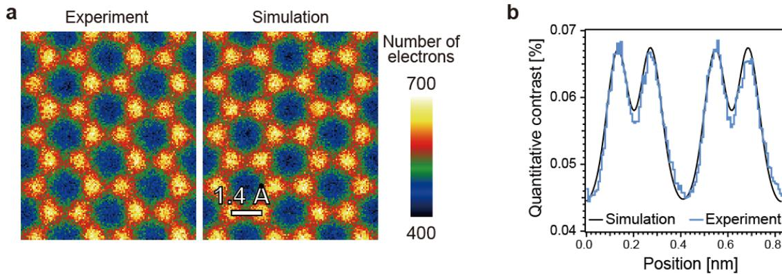
**Fig. 1 a** Quantitative ADF imaging of monolayer graphene. An experimental image was observed at 80 kV with a probe current of 27 pA. Multiple fast acquisition and drift correction were performed. Simulation includes residual aberrations, defocus spread and an effective source distribution, and the quantum noise is added on the basis of the Poisson process [4]. **b** Quantitative comparison between experiment and simulation that without the quantum noise.
