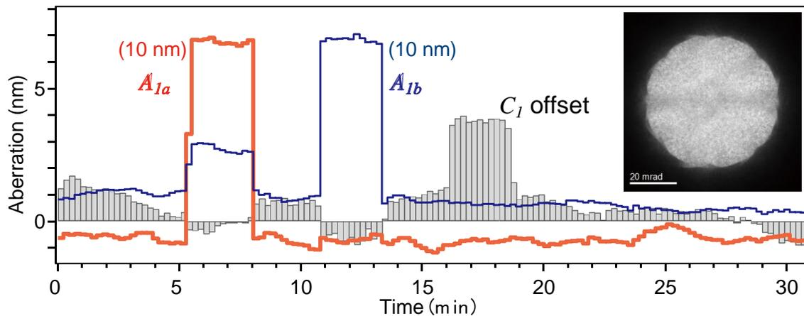
**Fig 2.** Time dependence of defocus  $C_1$  and two-fold astigmatism  $A_1$  as measured using our method [8]. A specimen was a  $\text{SrTiO}_3$  (001) film and the inset shows an experimental Ronchigram.
