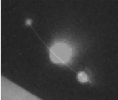
**A** Real-space optical image showing light emission from wire ends superimposed on a high-resolution SEM image of the silver nanowire
