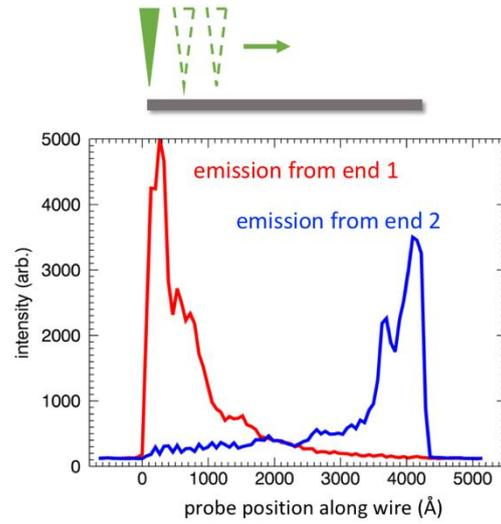
**B** Light emission from wire ends as a function of probe position
