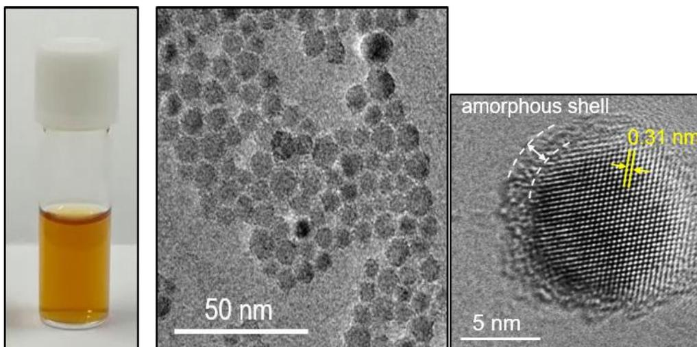
Figure 2. High-resolution TEM image of a codoped Si QD on graphene oxide film.
