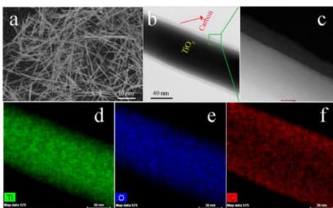
Figure . (a) SEM image of TiO<sub>2</sub> NWs; (b) BF-STEM image of the single core-shell structured TiO<sub>2</sub>@C-15 NW hybrid; (c) HAADF-STEM image of the corresponding enlarged region indicated by the green rectangle in part b; (d-f) EDS elemental maps of Ti, O, and C, respectively.
