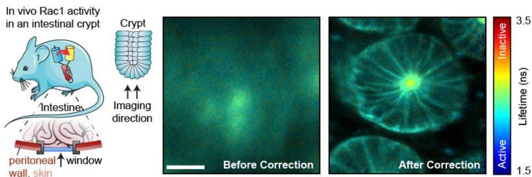
Figure 1. FLIM of intestinal crypts from the Rac1-FRET biosensor mouse in vivo using an abdominal titanium imaging window (left). Example intensity merged lifetime images (middle) before and (right) after motion compensation. White scale bar, 50  $\mu\text{m}$ .
