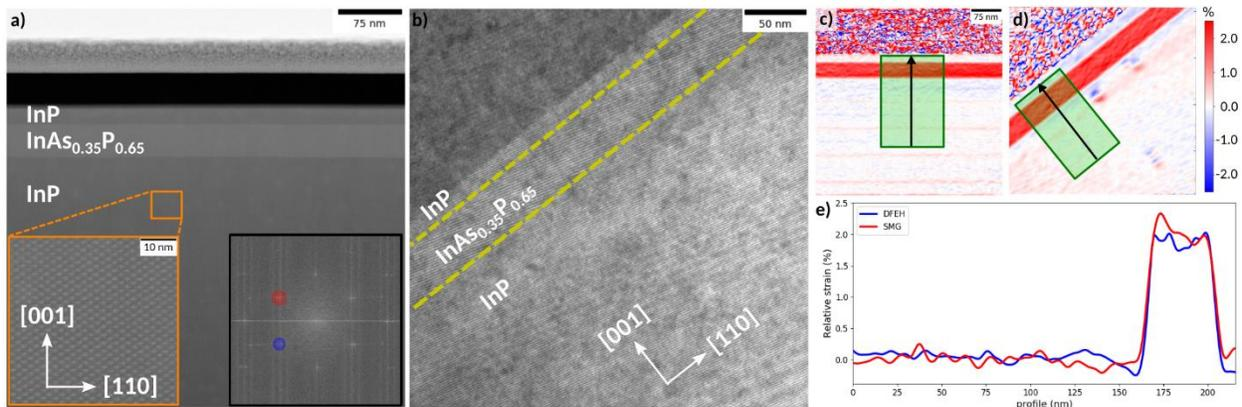
**Figure 1:** Strain characterization results on a InP/InAs<sub>0.35</sub>P<sub>0.65</sub>/InP sample. a) STEM Moiré hologram recorded using a pixel size of 0.466 nm. The bottom left inset corresponds to a digital zoom of the
