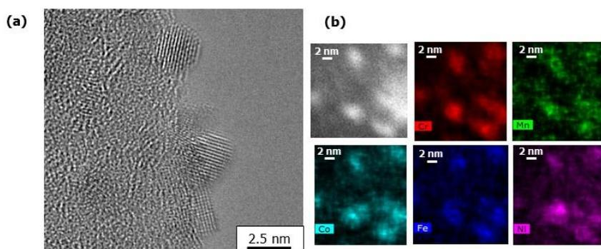
Figure 1: (a) Cs corrected high-resolution TEM image of high entropy alloy nanoparticles after their ex-situ crystallization (b) EDS elemental mapping for high entropy alloy nanoparticles after their in-situ TEM crystallization
