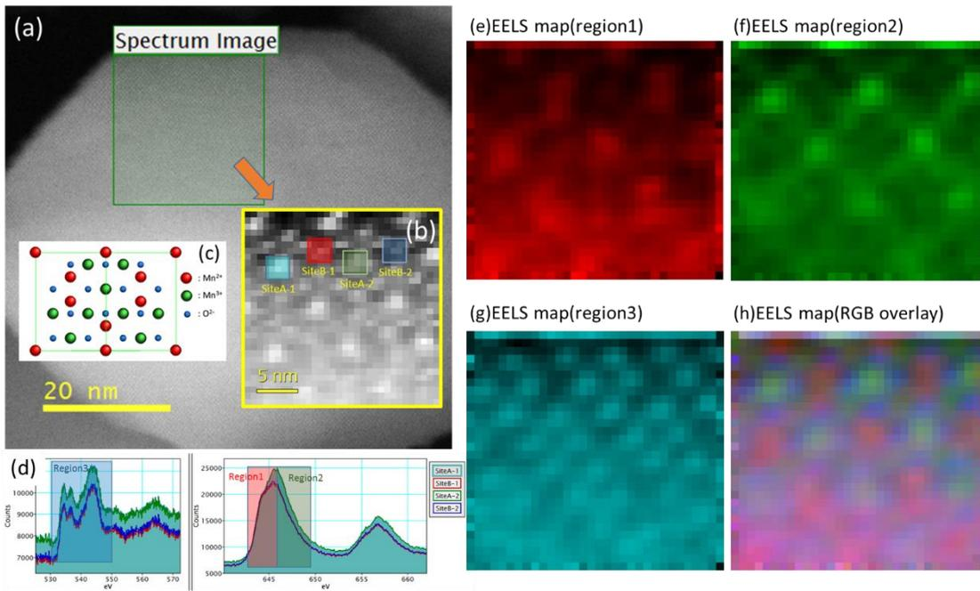
Figure. Mapping of a single crystal of Mn<sub>3</sub>O<sub>4</sub> by STEM moiré method.
