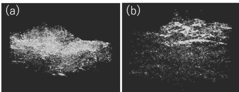
Figure 1 3D void configurations of non-heat-treated (a) and annealed composite electrode (b), respectively.
