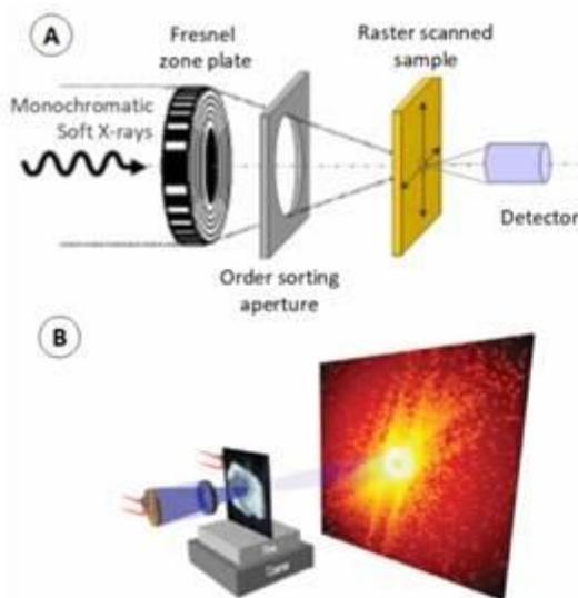
Fig. 1 Schematic of (a) STXM and (b) ptychography.
