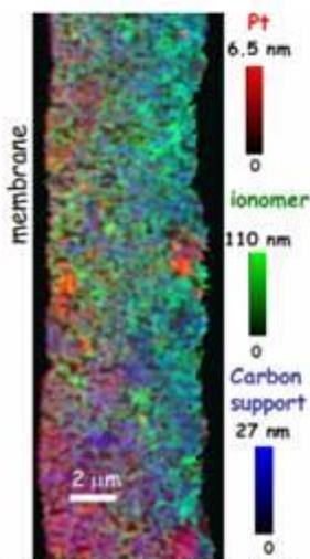
Fig. 2 Color coded composite of quantitative 2D projection maps of Pt, ionomer and carbon support in a PEM-FC cathode, derived from C 1s and F 1s STXM.
