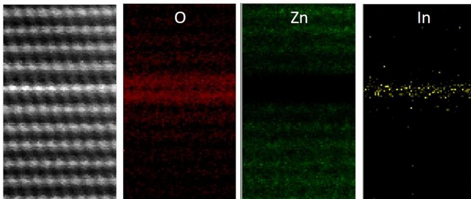
Figure 2. Atomic-resolution EELS mapping image of Zn and In element.
