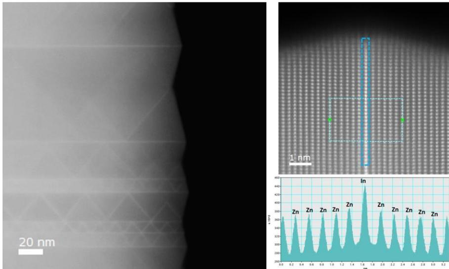
Figure 1. Atomic-resolution and low magnification HAADF-STEM image; columns of Zn and In cations are clearly resolved; weak signals from oxygen are not detectable.
