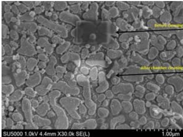
**Figure 1.** Specimen EBID before/after a SEM chamber was cleaned with the electron based cleaner
