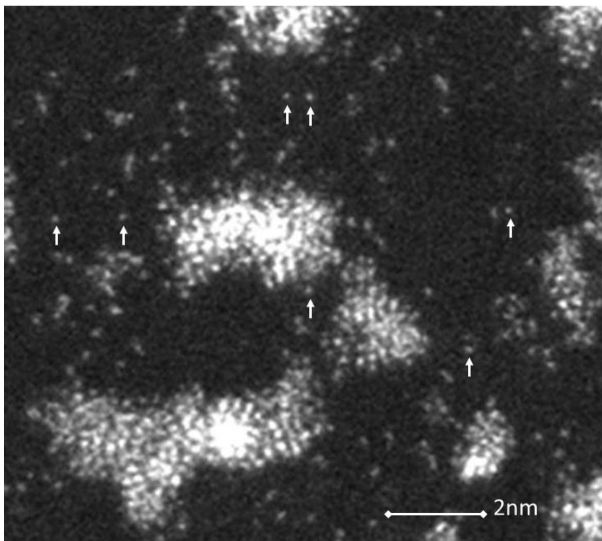
Fig.1: Single atom resolution ESTEM HAADF image of single atoms (a few are arrowed) individually isolated on the support on statistical kinetics or systematic pinned site basis, clusters and nascent partly crystalline particles of Pt on a carbon support film in the early stages of sintering in a 3Pa flowing H<sub>2</sub> environment using a modified furnace hot stage with replacement low noise electronics.
