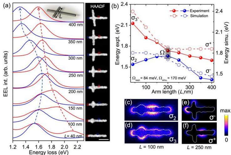
Figure 1. (a) EELS spectra for different crosses (see dark field image in inset, scale bar is 200 nm) taken at positions indicated by blue and red squares. (b) Experimental and simulated energy of the modes in a) as a function of the arm length  $L$ . Experimental energies have been deduced by Gaussian fit. (c-d) EELS filtered maps measured at energies corresponding to an uncoupled case for  $L = 100$  nm. (e-f) EELS fitted maps for the coupled case at  $L = 250$  nm
